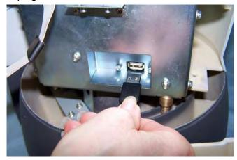
10. Remove the screws from the USB connector and remove it.
